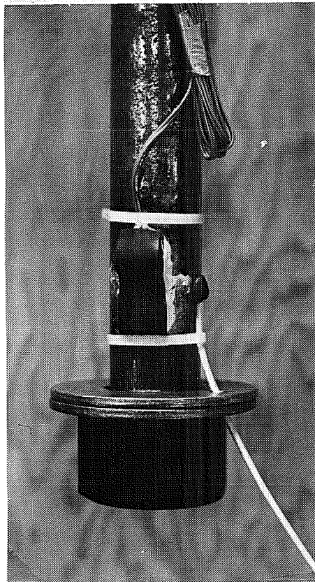
Fig. 2.15 (a) Lead slip wire; (b) tail slip wire and strain gage at the anchorage end.
